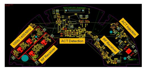
Fig. 4: RF PCB Layout
