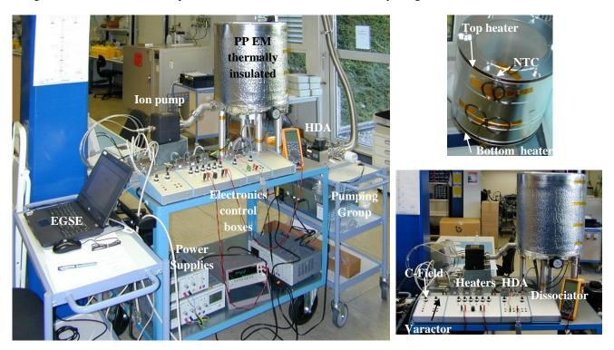
Fig.2: Technological Model Set-up and cavity view (top right)
