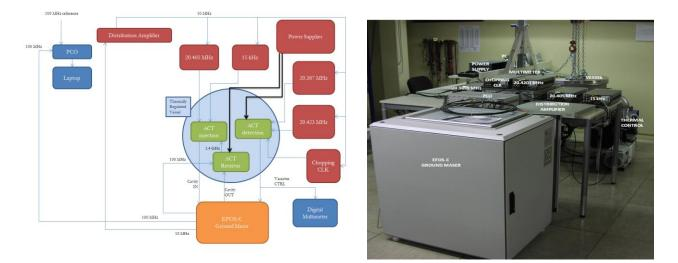
Fig. 5 : ACT validation test bench layout (left) and view (right)
